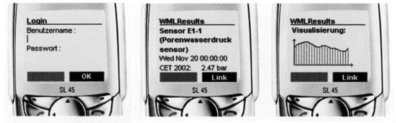
**Figure 3:** Informing the dam technician by mobile phone
