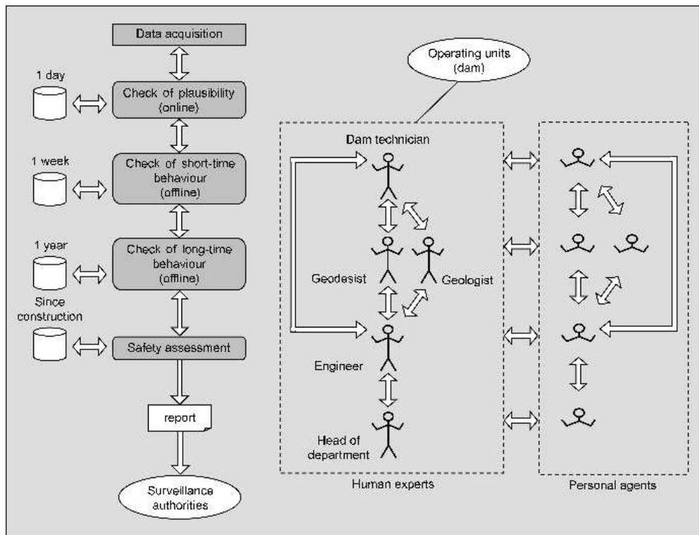
**Figure 2:** Conceptual design of dam monitoring
