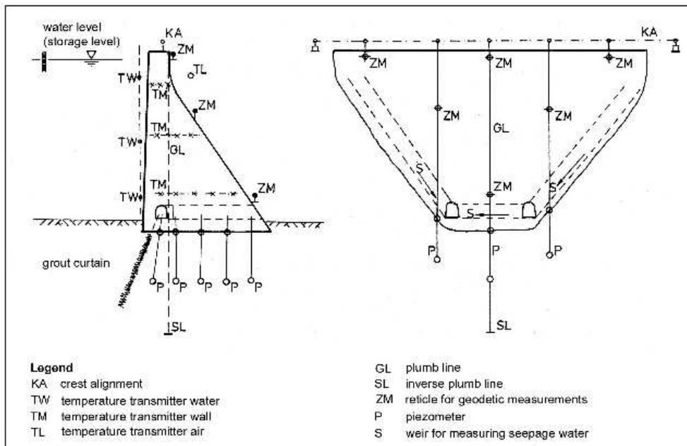
**Figure 1:** Example for the configuration of measuring devices [1]
