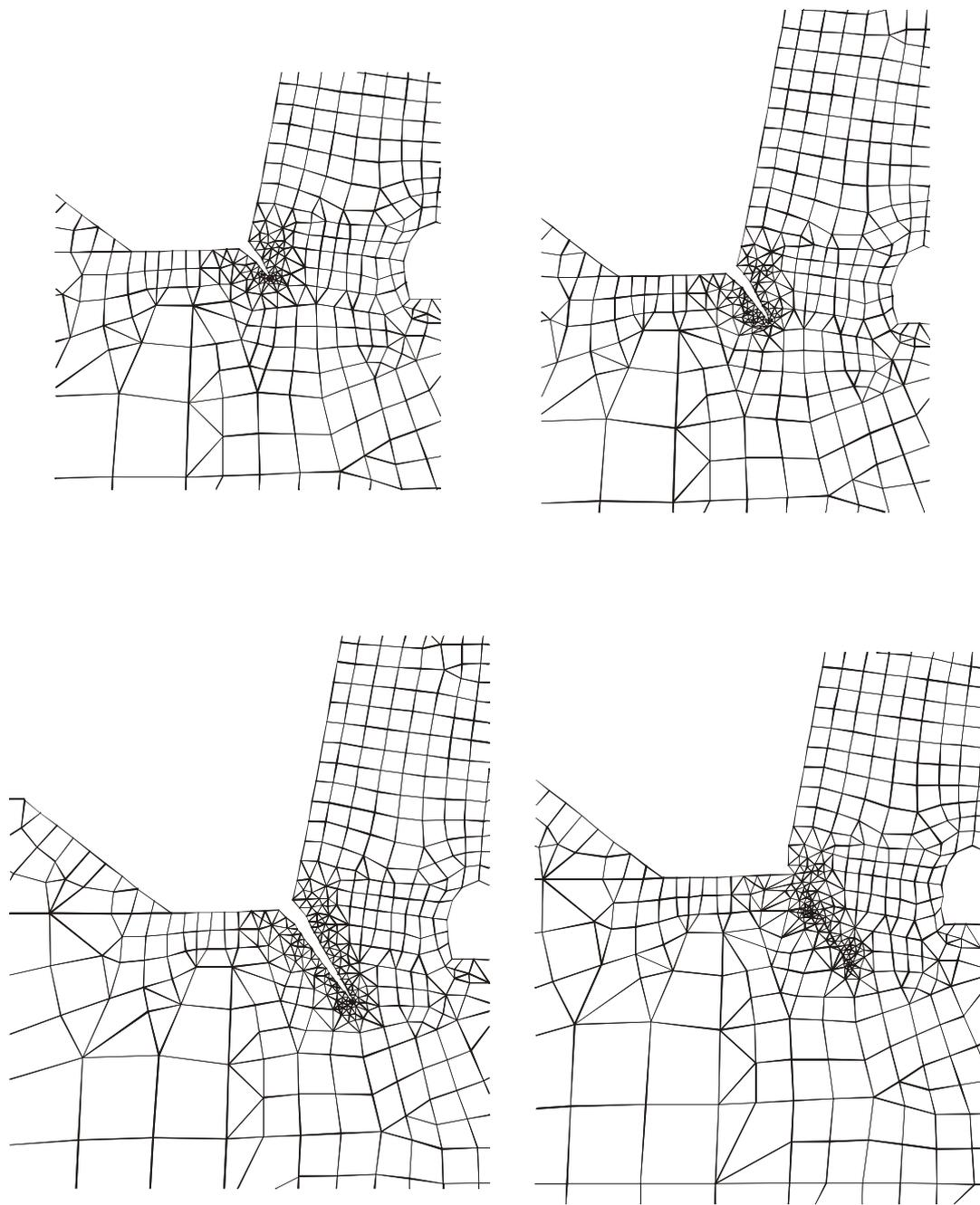
Figure 5. Displacement conditions during crack propagation
