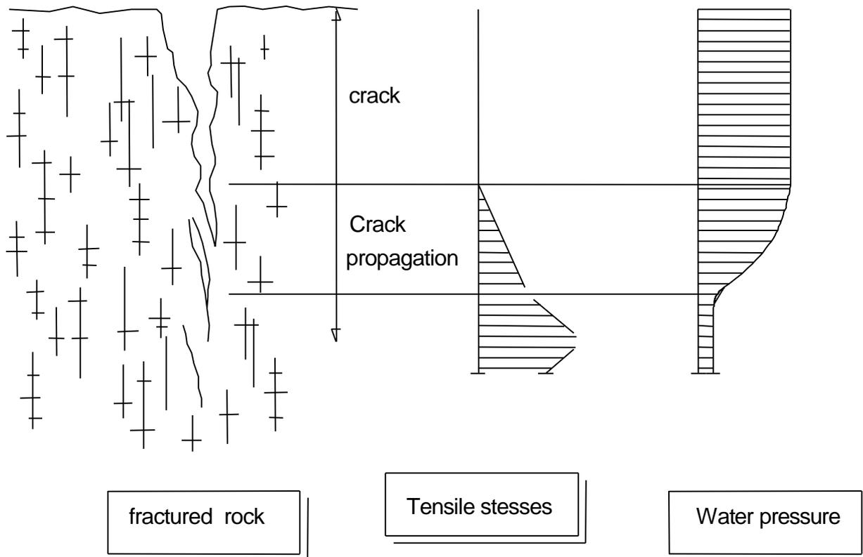
Figure 2: Process of the crack propagation
