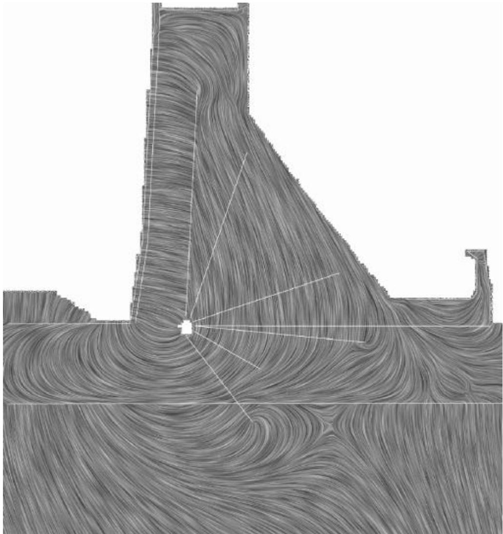
Figure 4. Seepage within the dam
