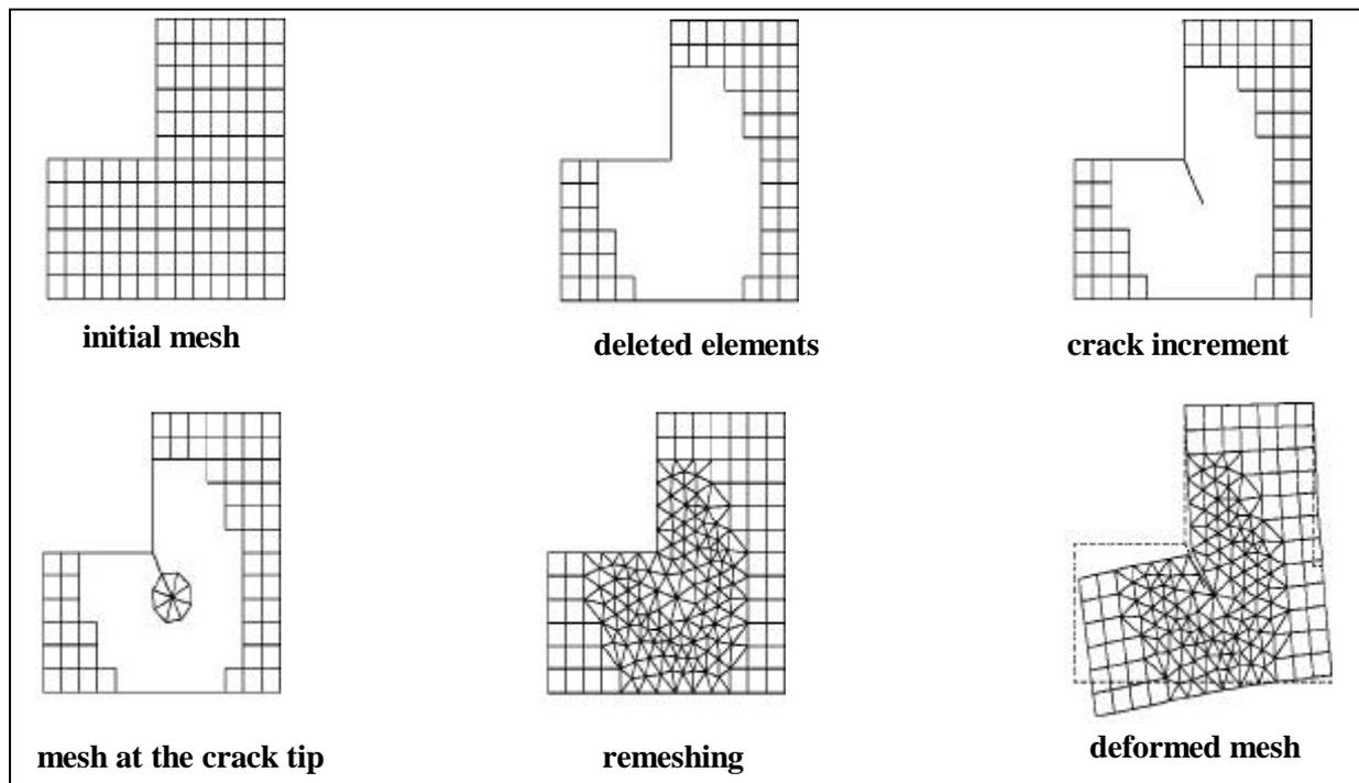
Figure 3: Remeshing Procedure to simulate a discrete crack
