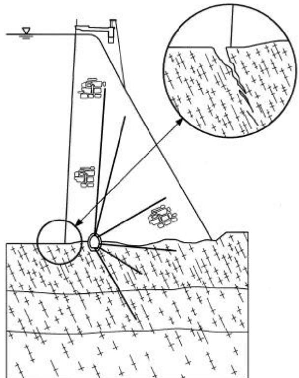
Figure 1. Crack in dam foundation
